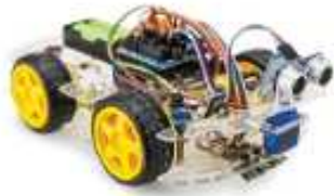
Programmable 4 wheel drive robotic car
