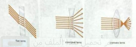
A. Which lens makes the light's path shifts a little, but its final direction does not change?
